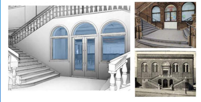
Restoration of the exterior stairs case & community room entrance
